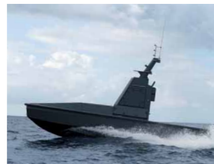
The Venus Unmanned Surface Vehicle is re-configurable for multi-missions
